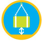
b) any bond between the load and its support, causing resistance when lifting the load
