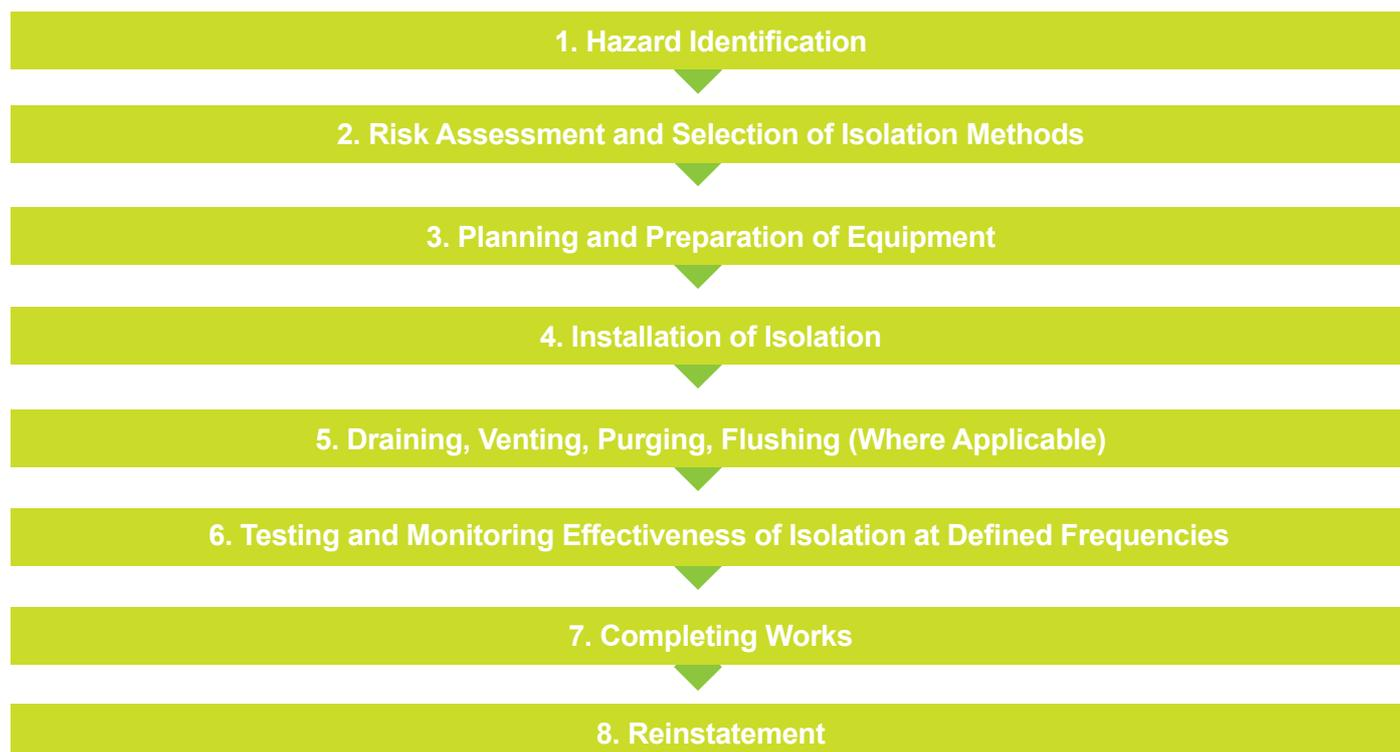
Fig 1. Safe isolation procedure
