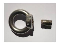
A dangerous occurrence has recently been recorded in relation to the failure of a removable lifting eye whilst a lifting operation was being carried out on a 371kg sluice valve. The failure was immediate and approx. 6" off the lifting surface and no injuries were recorded, however the consequences could have been for more severe.
