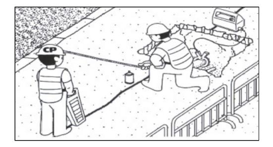
When excavating for existing services, the trial hole must be carried out by hand, mechanical and power tools must never be used directly over an existing service, as this may result in a fatal explosion or electrocution.
