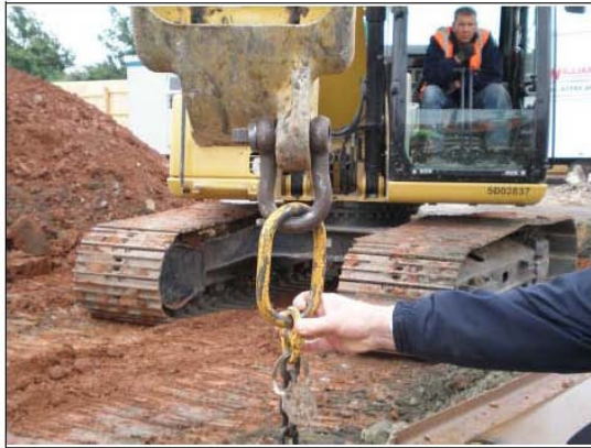
Figure 1 - Master link rotation restricted to approx \pm 70^\circ
