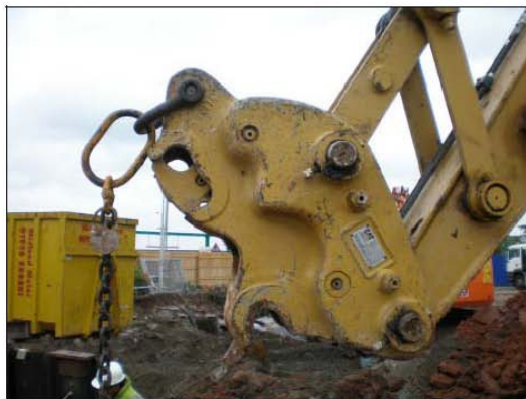
Figure 3 – Hitch tilted backwards with master link subject to bending
