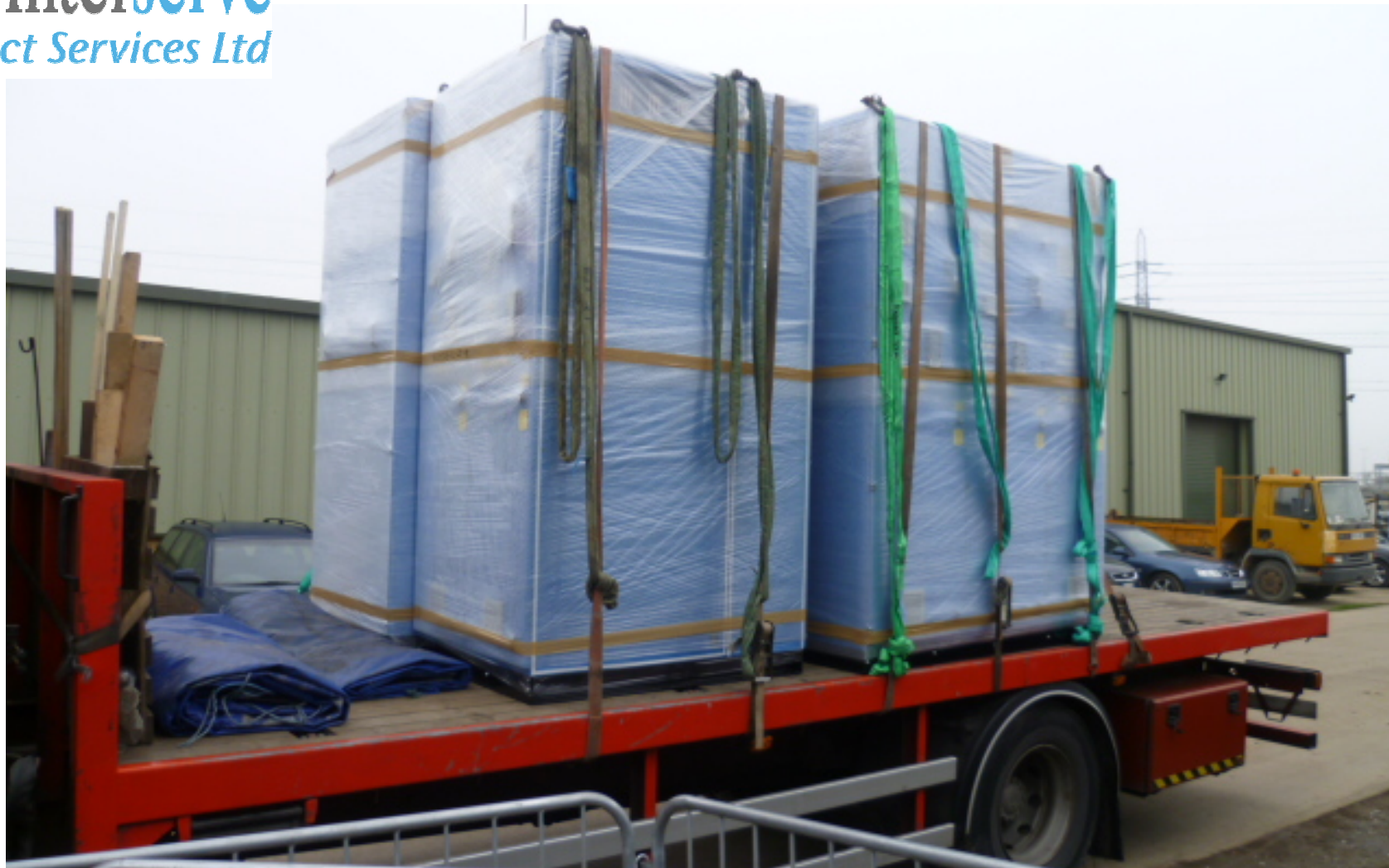
MCC Panels, delivered to Riverside, ready for safe unloading without the need for anyone to climb up onto the wagon.
