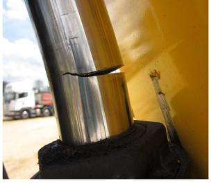
Thankfully the operator of the excavator had lowered the load to the ground when the failure was identified and the machine immediately quarantined. However, if the boom had completely failed and the load dropped during the lift, this could have resulted in far more serious incident.
