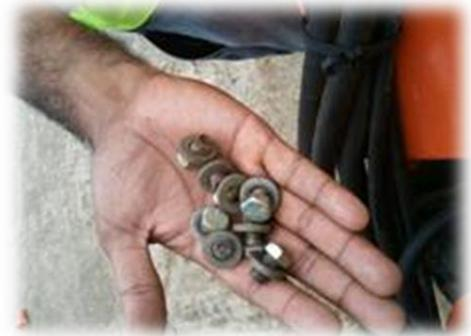
**Statement:** A JLG model 860SJ aerial lift was found to have all eight of its platform rotator attachment bolts sheared in half. This condition is not obvious during a visual inspection. Although there was no risk of the platform detaching from the boom the horizontal rotation capacity of the platform was severely compromised.
