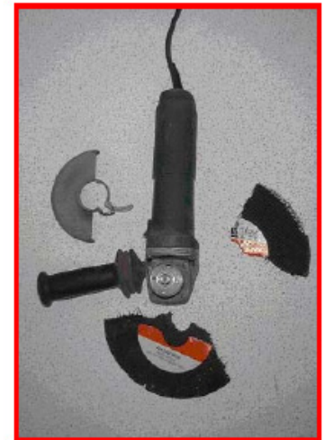
Angle grinder and disintegrated disk
