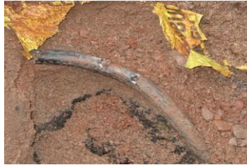
P3 Spade Damage x2
