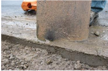
P1 Damage to the Spade
